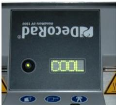
Switch off the UV lamp when ready. The text COOL will be shown.
