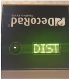
DIST = distance to surface is not correct / unsafe, a beeping signal can be heard
