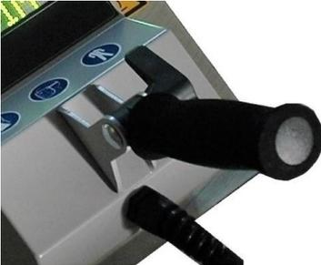
Adjust the (optional) extension pole. (or the small handle; not necessary to connect the data cable, use the button on the lamp unit – small handle has no data cable!)
