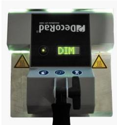
The beeping signal will stop if a safe distance is reached, the text DIM will be shown
