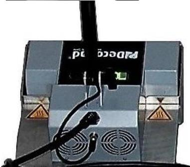
Connect the data cable of the extension handle to the back of the lamp unit
