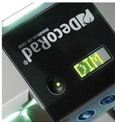
Use the button on the lamp unit or the extension handle to start UV curing
