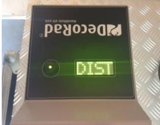
DIST = distance to surface is not correct / unsafe, a beeping signal can be heard
