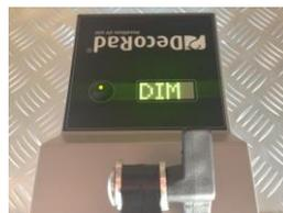
When DIM is shown in the display, the HandMate UV 600 is ready to use
