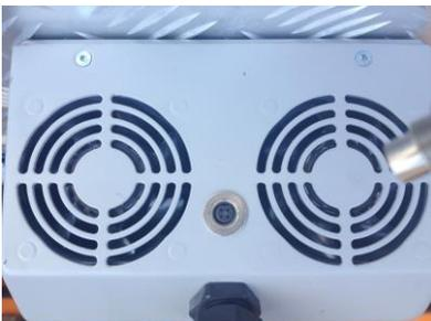
Connect the data cable of the extension handle to the back of the lampunit
