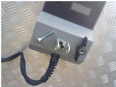
Adjust the (optional) extension handle (Or the small handle; not necessary to connect the data cable, use the button on the lamp unit – small handle as no data cable!)
