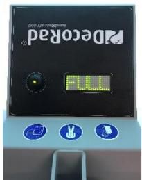
Use the button on the lampunit or the extension handle to open the shutter and to start UV curing. The text **FULL** will be shown on the display.
