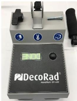
Optional: adjust the DecoRad® Handmate UV 600 extension pole. While using the extension pole, you need to connect the data cable with connector to the back side of the UV hand unit.
