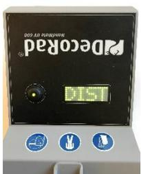
Move the lamp unit in a position between 2 – 4 centimeters from the surface. **DIM** will be shown on the display. The lamp can go to **FULL** and curing can be started again.
