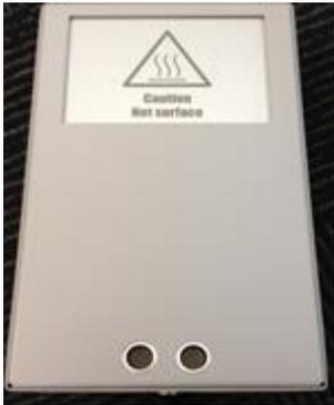
Shutter on the bottom of the Handmate UV 600.
